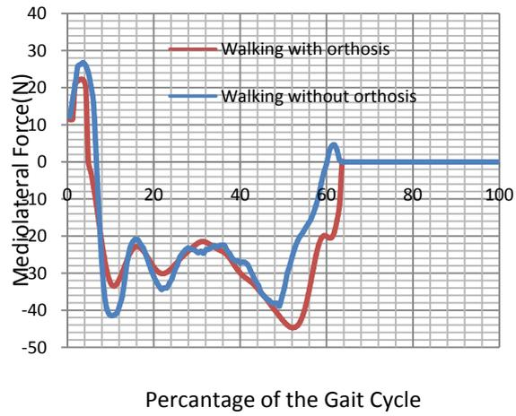
Figure 3: Medirolateral force applied on the limb while walking with and without orthosis (subject 1)
