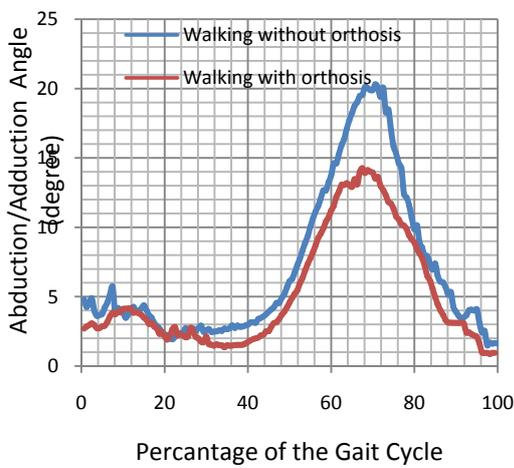
Figure 2: Abduction/adduction angle of the knee joint while walking with and without orthosis (subject 1)
