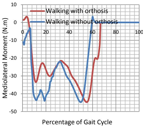
Figure 4: Medirolateral moment applied on the knee joint while walking with and without orthosis (subject 1)
