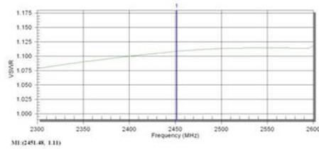
Figure 3: VSWR(Voltage Standing Wave Ratio) characteristic of open-tip bended antenna.
