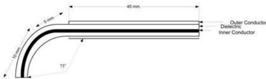
Figure 2: Antenna structure.
