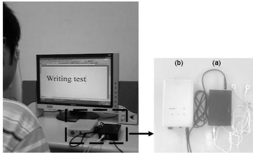
Fig. 5 The photograph of EMcTin and typing test by user: (a) EOG input interface (b) Morse code translate input device
