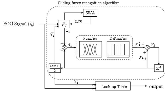
Fig. 3. The sliding fuzzy recognition algorithm [19]
