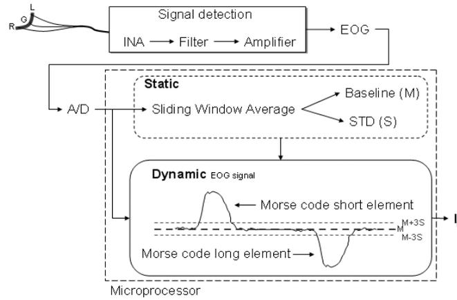
Fig. 2. The structure of EOG two switch
