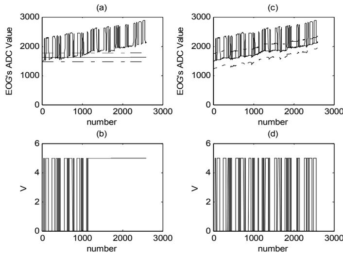
Fig. 4 The robust test of EOG input interface: (a) EOG sequences without baseline tracing algorithm (b) the recognition result without baseline tracing algorithm (c) EOG sequences with baseline tracing algorithm (d) the recognition result with baseline tracing algorithm
