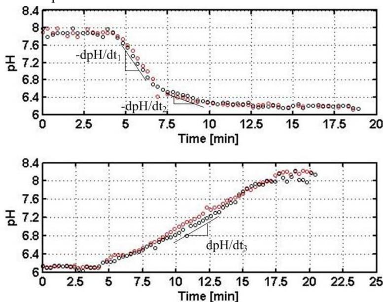
Fig. 3. Responses from the titration experiments. Top: YPD medium ( $\text{pH}_0 = 8$ ) titrated with  $\text{CO}_2$  gas (at 2 bar and  $25^\circ\text{C}$ ) to a final pH of about 6.3. Bottom: YPD medium ( $\text{pH}_0 = 6$ ) titrated with  $\text{NH}_3$  (20 000 ppm) –  $\text{N}_2$  gas mixture (at 1 bar and  $25^\circ\text{C}$ ) to a final pH of about 8.2.
