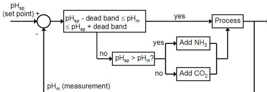
Fig. 1. Block diagram of the on/off pH controller.
