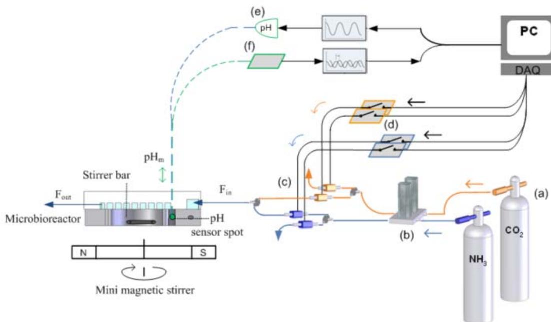
Fig. 2. Schematic of the gas connections for the gaseous pH control scheme. (a)  $\text{NH}_3$  and  $\text{CO}_2$  gas bottles (b) mass flow meters (c) solenoid valves (d) relays (e) LED (465 nm) (f) photo detector. Dashed lines (---), represent optical fibers, black solid lines represent electrical wiring (-), and blue/orange solid lines represent tubing for fluidics (-/-).
