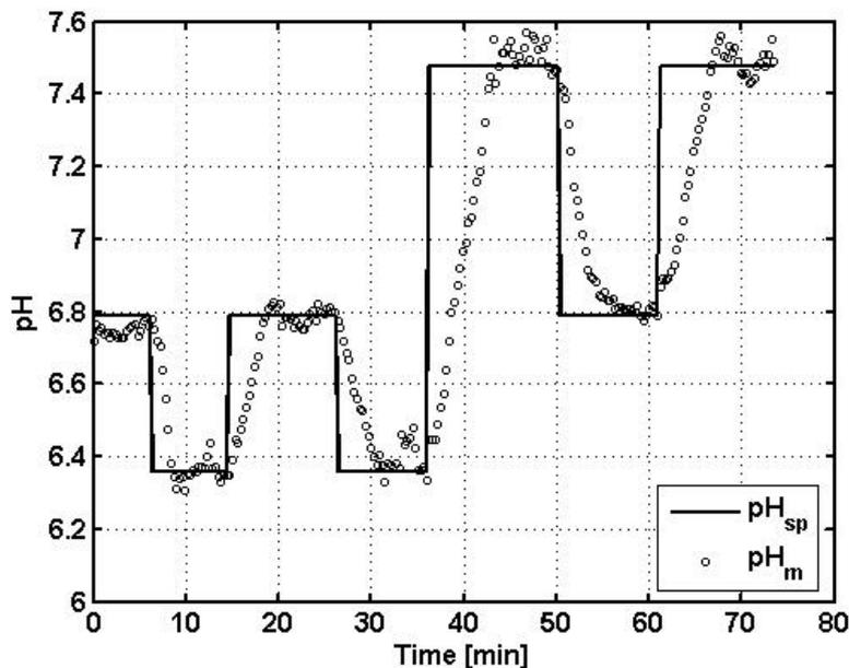
Fig. 4. Closed loop response of the on/off pH controller for different set point values ( $\text{pH}_{\text{sp}} = 6.8, 6.3$  and  $7.5$ ), starting from pH 6.8.
