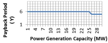
Fig. 4: PBP versus Power Generation Capacity
