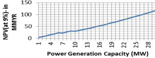
Fig. 3: TNPVI versus Power Gen. Capacity
