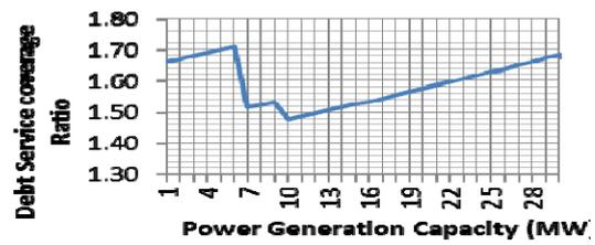
Fig. 2: DSCR versus Power Gen. Capacity
