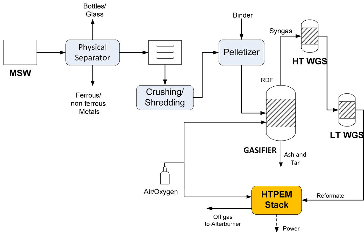
Fig. 1: The Proposed Cogeneration System
