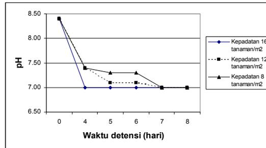
Fig. 2: PH in the reactor parameters with Papyrus Plant
