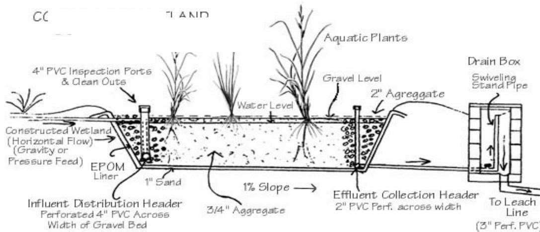
Fig. 1: Elongated pieces of artificial marsh reactor
