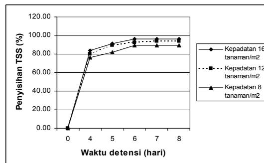
Fig. 4: Provision for TSS measurements in the reactor with Papyrus Plant
