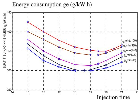
Fig. 3: relationship between energy consumption with injection time
