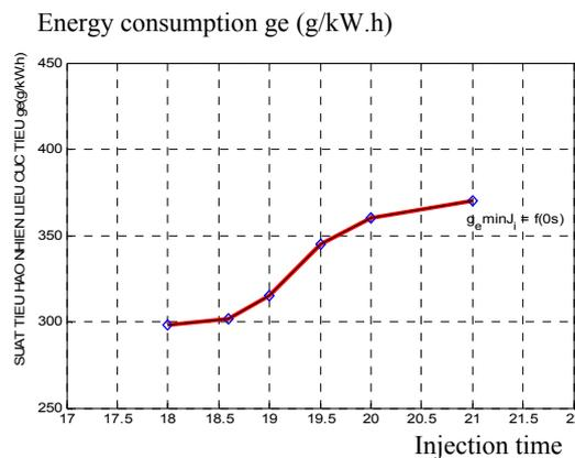
Fig. 4: relationship between minimum energy consumption with injection time
