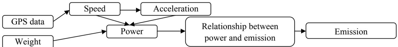
Fig. 6: Process of calculation emission
