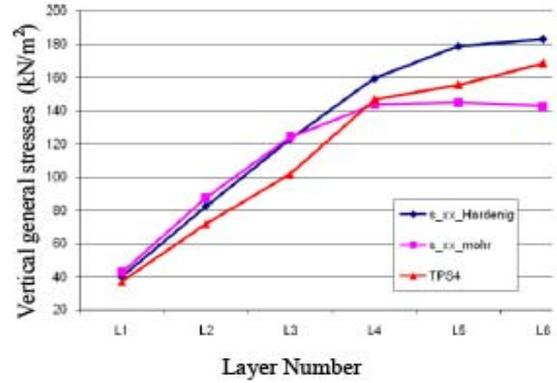
Fig. 4: Comparing the results of instrumentation TPC3 with those of Mohr-Coulomb and Hardening models for different stages of backfilling
