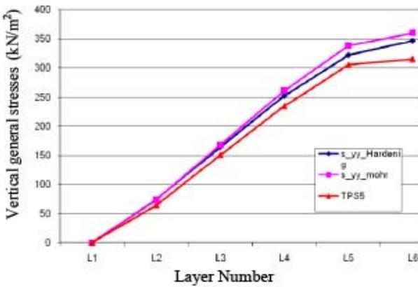
Fig. 5: Comparing the results of instrumentation TPC4 with those of Mohr-Coulomb and Hardening models for different stages of backfilling
