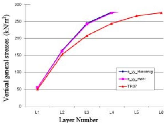
Fig. 7: Comparing the results of instrumentation TPC6 with those of Mohr-Coulomb and Hardening models for different stages of backfilling
