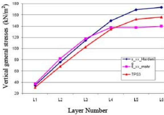
Fig. 3: Comparing the results of instrumentation TPC2 with those of Mohr-Coulomb and Hardening models for different stages of backfilling
