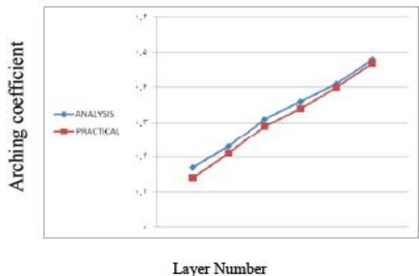
Fig. 8: Comparing the results of instrumentation TPC7 with those of Mohr-Coulomb and Hardening models for different stages of backfilling
