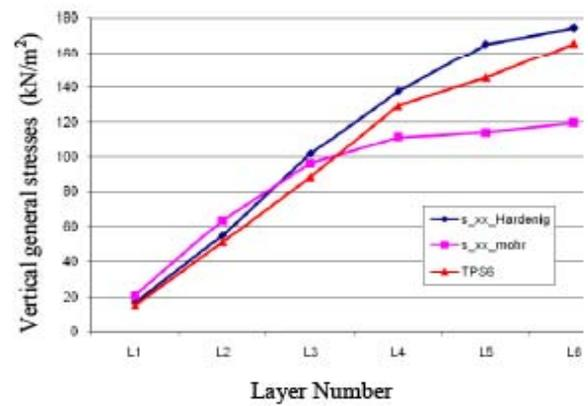
Fig. 6: Comparing the results of instrumentation TPC5 with those of Mohr-Coulomb and Hardening models for different stages of backfilling
