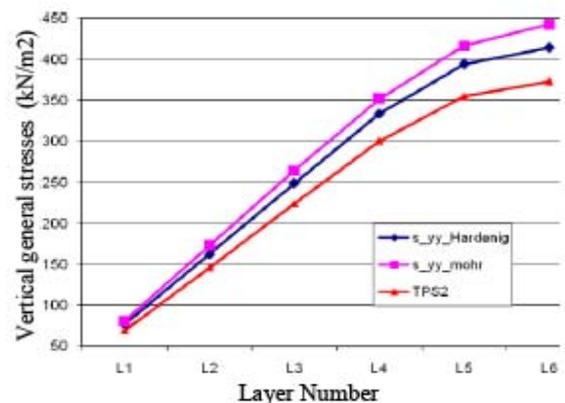
Fig. 2: comparing the results of instrumentation TPC1 with those of Mohr-Coulomb and Hardening models for different stages of backfilling
