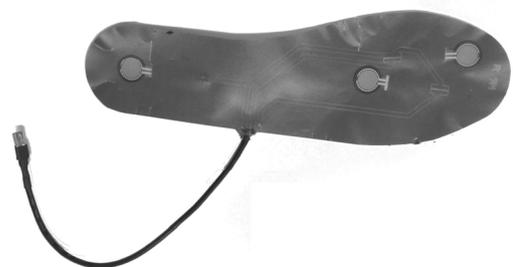
Fig. 2: Flexible insole with pressure sensors
