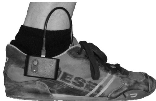
Fig. 1: Sensor array mounted on shoe
