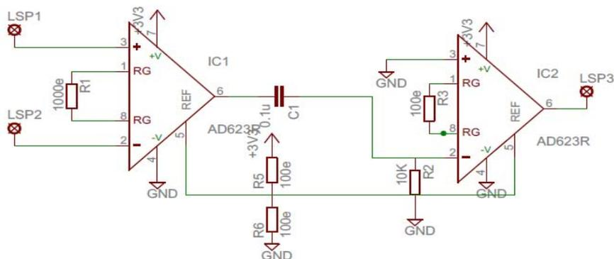
Fig. 2: Schematic of preamplifier unit
