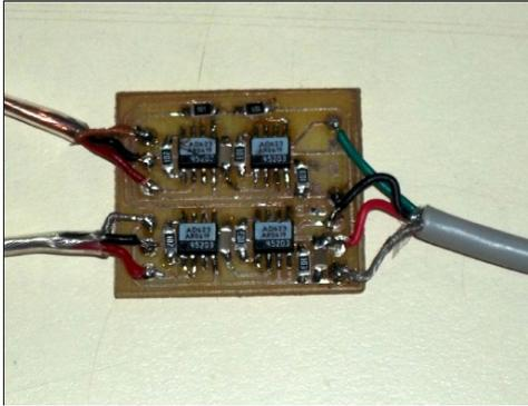
Fig. 3: Preamplifier board
