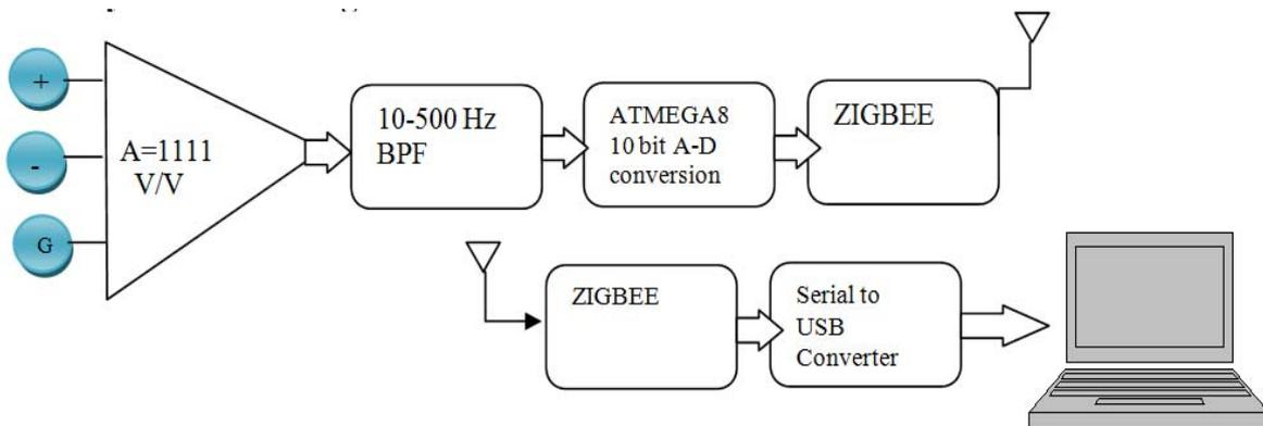
Fig. 1: EMG system block diagram
