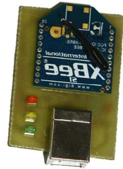
Fig. 5: USB Xbee Transceiver
