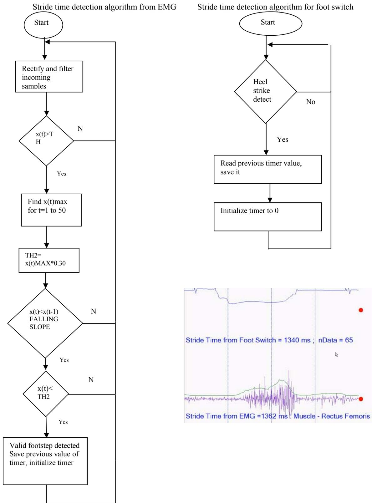
Fig. 7: Snapshot of the acquisition window. Switch Waveform (top) and EMG waveform (Bottom).
