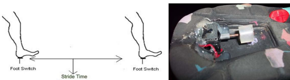
Fig. 6: Foot switch attached beneath shoe
