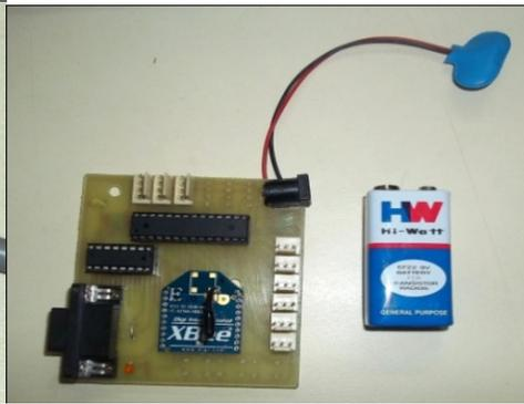
Fig. 4: Microcontroller and XBee
