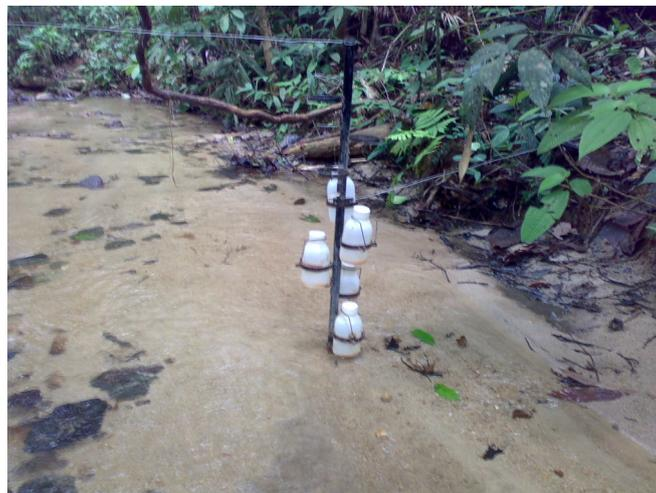
Figure 2. A multi-stage of sediment sampling during storm equipped with bottle of 10-cm interval as water level.
