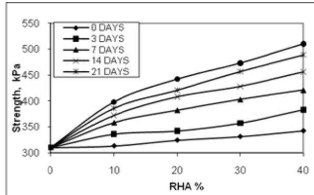
Fig 2: Variation of strength of B C soil on addition of RHA
