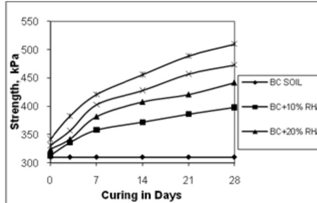
Fig 5: Variation in strength of B C soil upon curing
