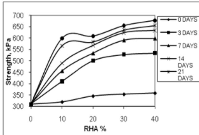
Fig 3: Variation of strength of B C soil on addition of RHA and 3% lime
