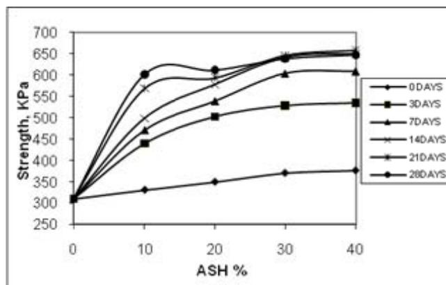
Fig 4: Variation of strength of B C soil on addition of RHA and 5% lime
