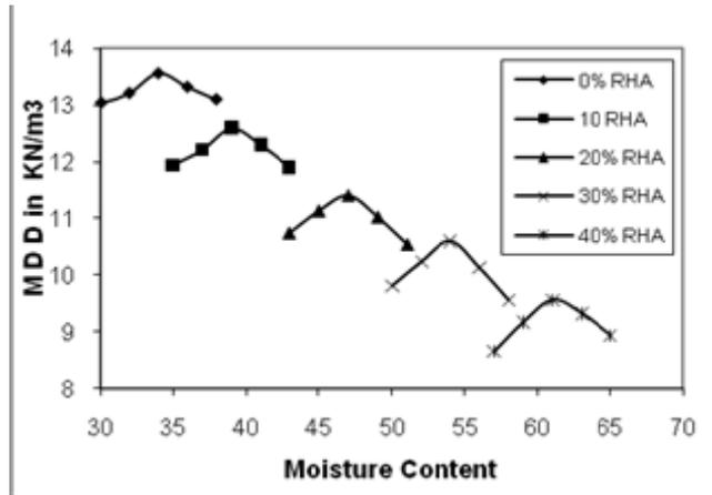
Fig 1 : Compaction curves of B C soil and RHA mixtures
