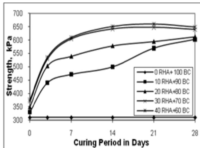
Fig 6: Variation in strength of B C soil, RHA and 5% lime upon curing
