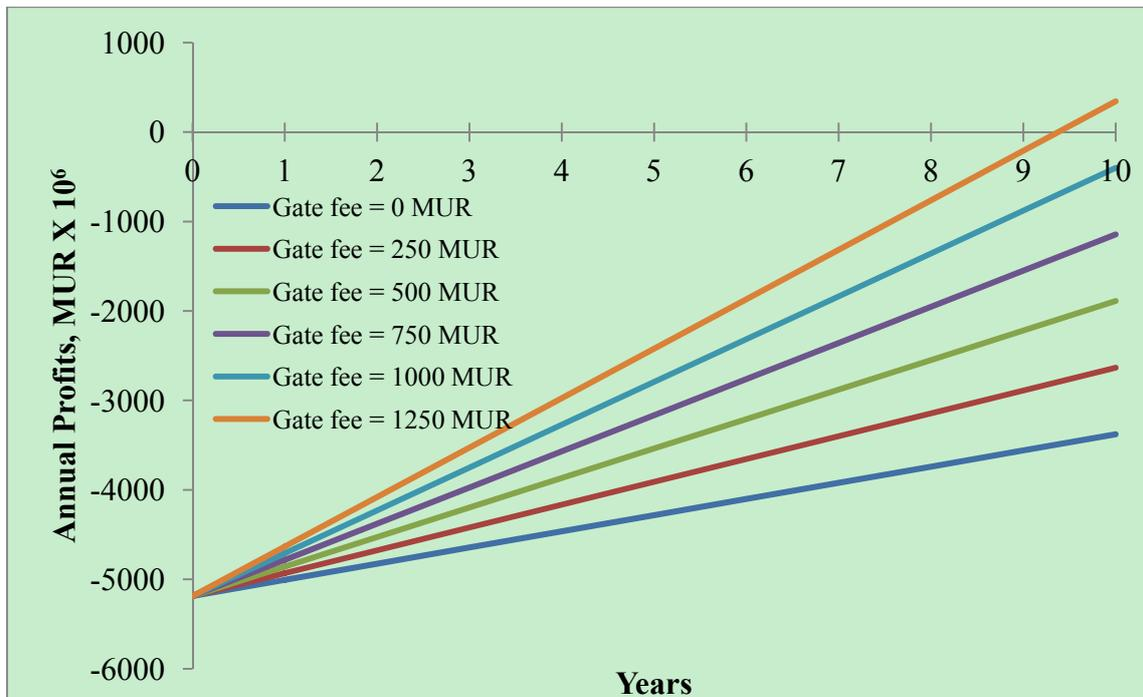
Fig. 1: Annual profit for biogas to energy plant
