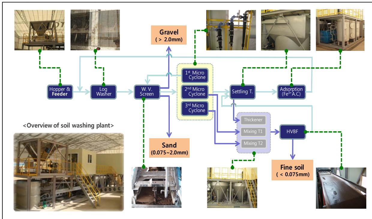
Fig. 2: Description of soil washing process and main facilities
