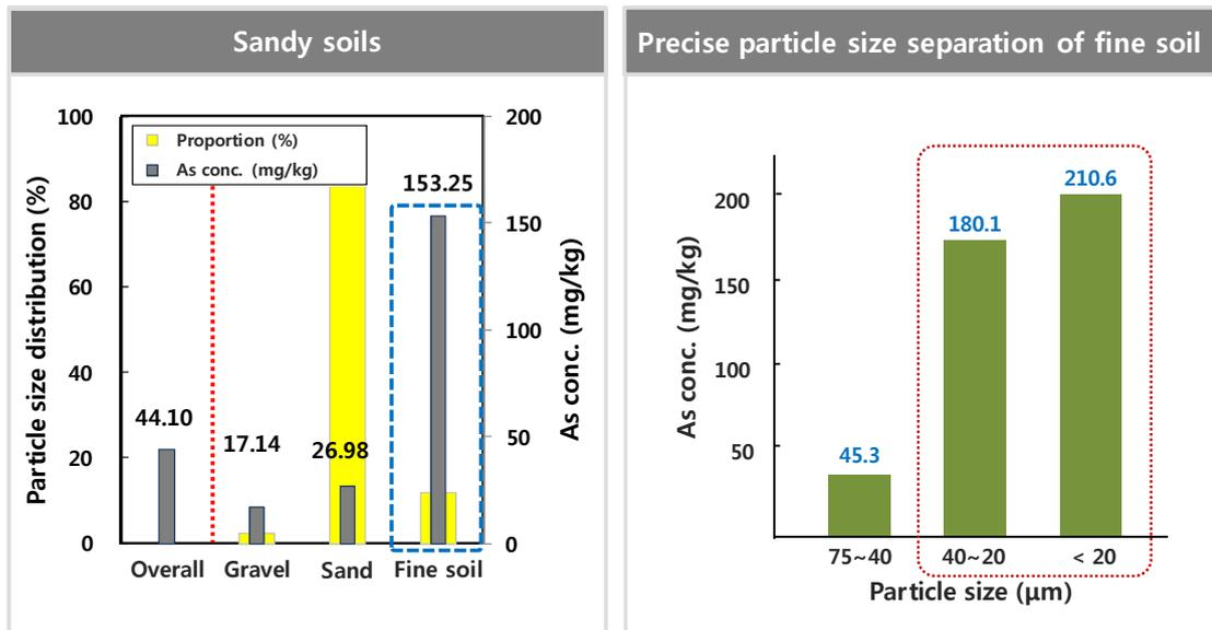
Fig. 4: Contamination distribution of sandy soils by particle-size separation
