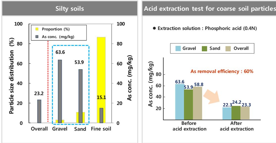
Fig. 5: Contamination distribution of silty soils by particle-size separation
