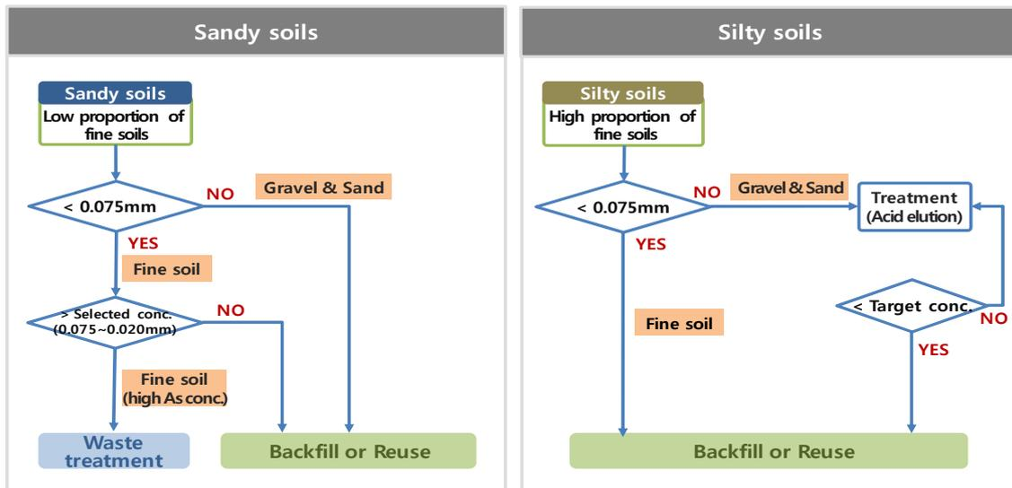
Fig. 6: Remediation process according to the soil texture
