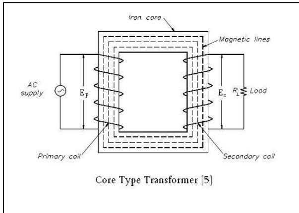
Assuming ideal transformer action, the voltage in the secondary winding  $E_s$  and the voltage in the primary winding  $E_p$  are related as in (1). [6]
