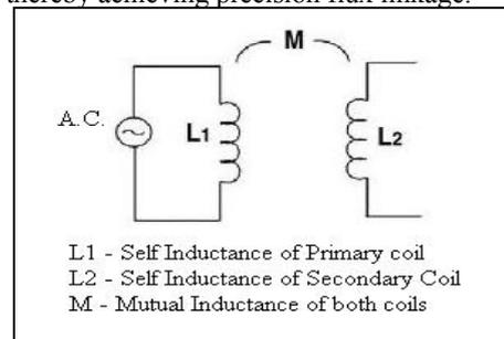
However, its short range is a cause of concern as the separation between the two inductive coils is placed very close to each other. Considering its commendable efficiency during power transmission it is used for wireless charging of electrical and electronic devices and one such example is electronic truth brushes.
