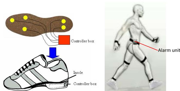
Fig. 2: Layout of the prototype for insole-feedback shoes.
