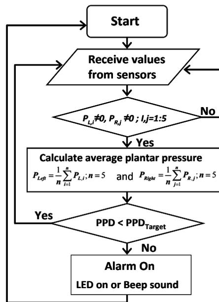
Fig. 3: Flow chart of data processing for insole feedback.
