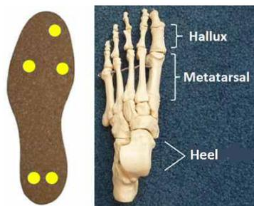
Fig. 1: Positions of FSR under the insole.
