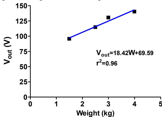
Fig. 6: The relationship between testing weights and output voltages of the controller box
