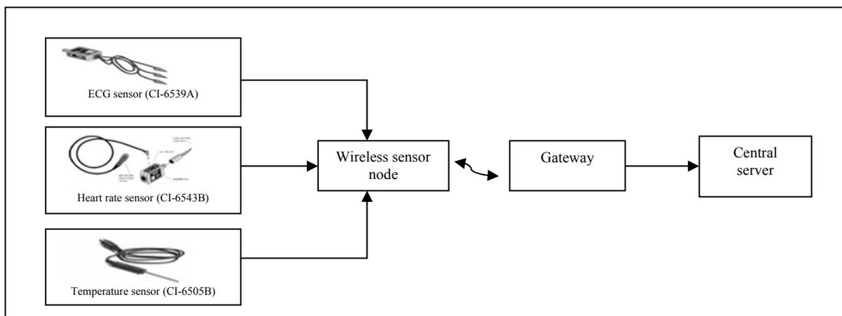
Fig 2: Wireless sensor node Interfaced with Physiological Sensors and the central server
