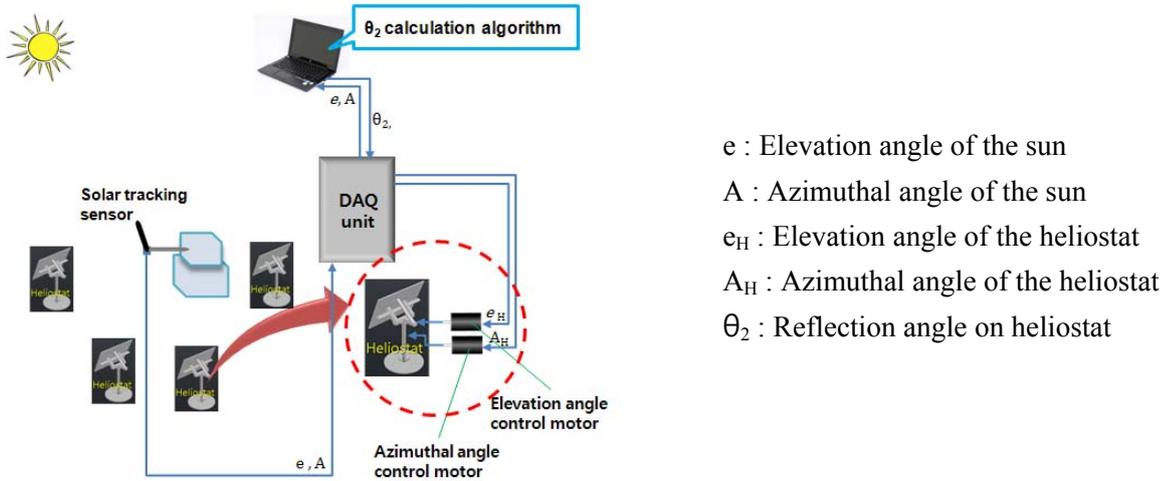
Fig. 3: Control algorithm
