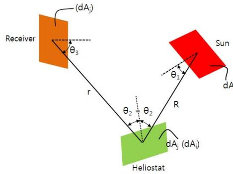
Fig. 2: Schematic diagram of two configuration factors
