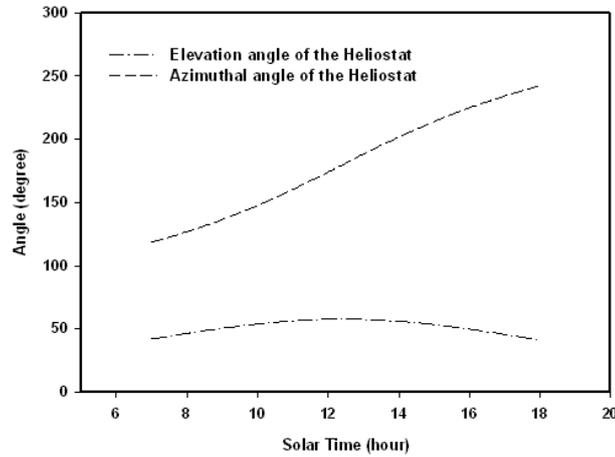
Fig. 7: Elevation and azimuthal angle of the heliostat versus solar time, season: spring or autumn, distance: 50m
