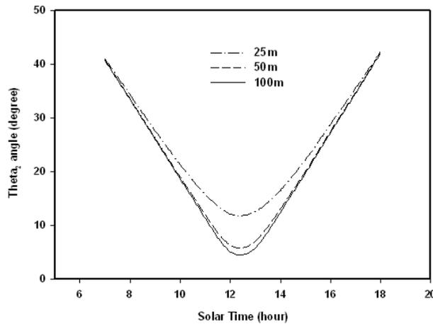
Fig. 5: Incidence angle versus solar time for different distances from receiver to heliostat (spring or autumn)
