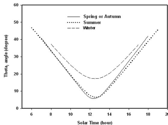
Fig. 6: Incidence angle versus solar time for different seasons, distance: 50m
