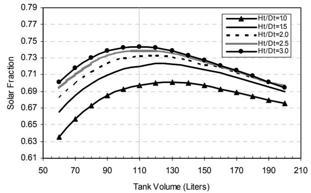
Figure 10 Effect of tank volume on solar fraction when the daily draw is 180 lit
