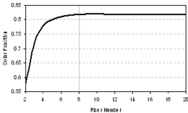
Figure 3 Effect of number of risers on the system solar fraction
