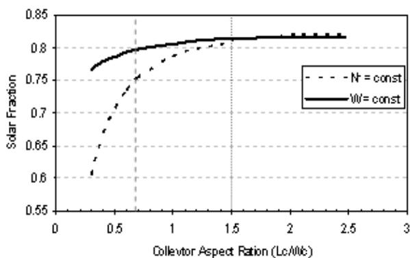
Figure 5 Effect of changing aspect ratio of the collector on the solar fraction
