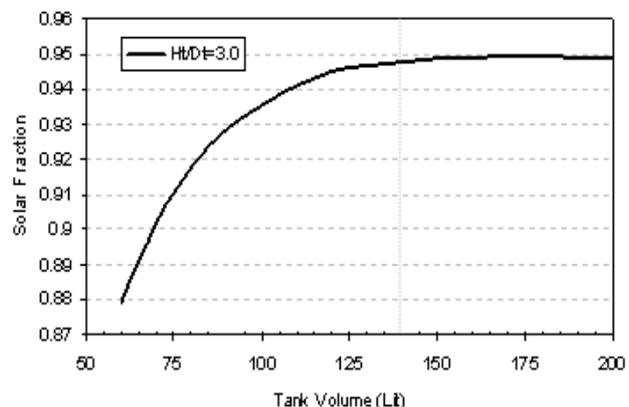
Figure 12 Effect of tank volume on solar fraction when the area of the system is doubled
