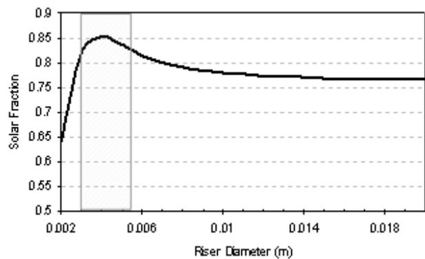
Figure 4 Effect of riser diameter on the system solar fraction
