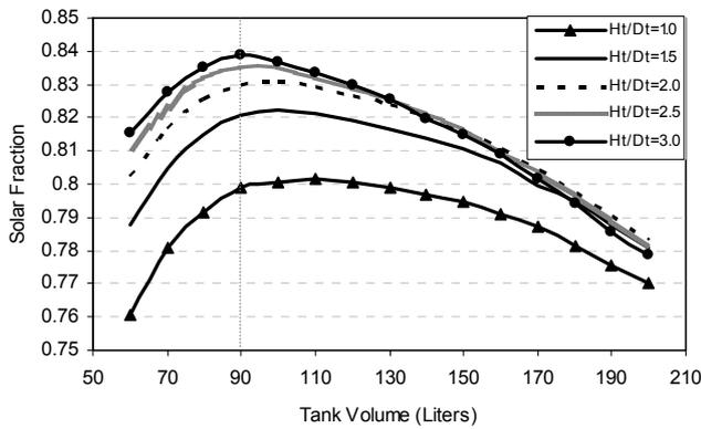
Figure 9 the effect of tank volume on the system solar fraction
