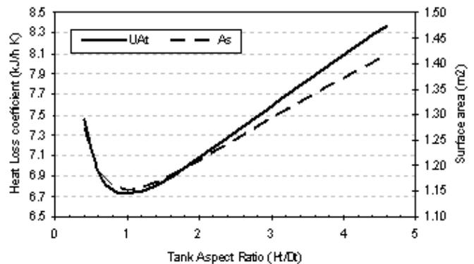
Figure 6 effect of aspect ratio on the heat loss coefficient
