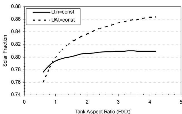
Figure 7 Effect of the tank aspect ratio on the solar fraction of the system
