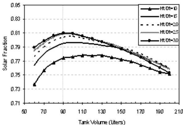
Figure 11 Effect of tank volume on the system solar fraction at different tank aspect ratio
