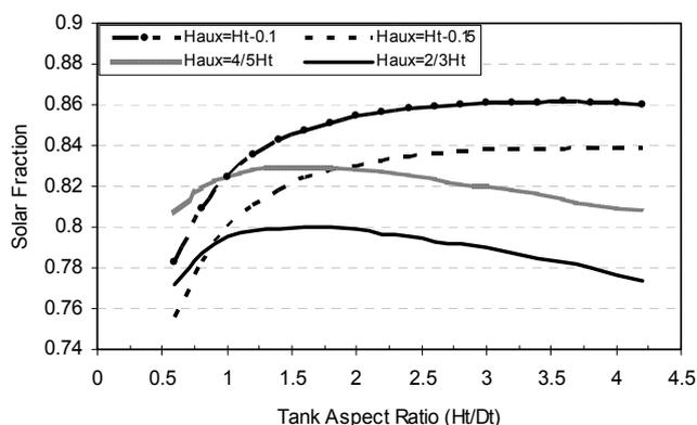
Figure 8 Effect of the tank aspect ratio on the solar fraction of the system
