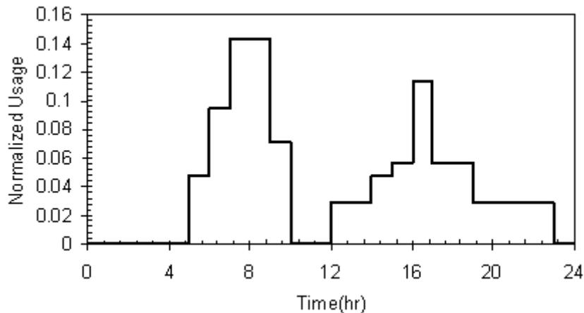
Figure 2: Hot water load pattern used for the study
