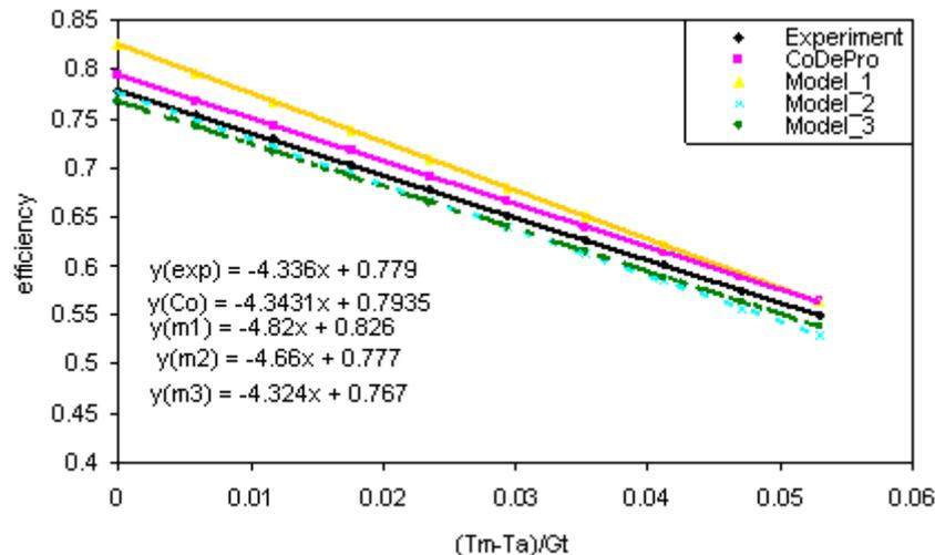
Figure 2: Experimental and theoretical efficiency curves for collector 1
