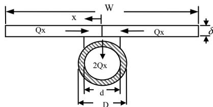
Figure 1: Fin and tube cross section
