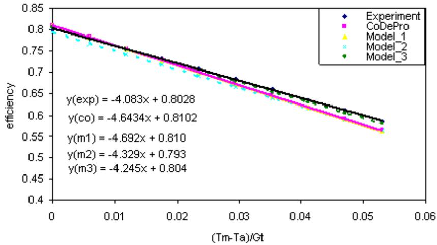
Figure 3: Experiment and theoretical efficiency curves for collector 2
