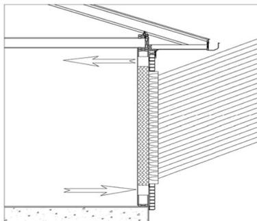
Fig. 4: Solar Air Collector
