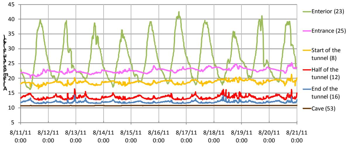
Fig. 2: Evolution of air temperatures inside the entrance, tunnel and cave, in the middle of August.
