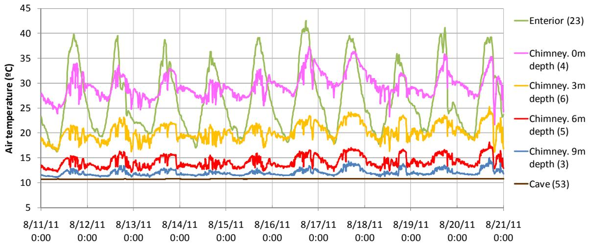
Fig. 3: Evolution of air temperatures inside the ventilation chimney and cave, in the middle of August.
