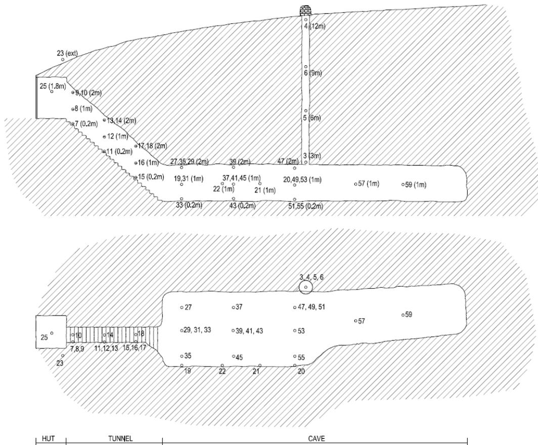
Fig. 1: Elevation and layout of the underground construction. Position and height of the sensors.
