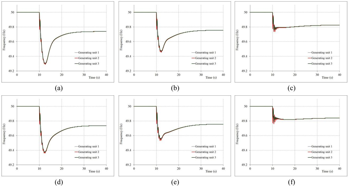
Fig 2. System frequency by different penetration index (PI) and different dependency to the frequency distortion
