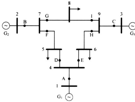
Fig 1: Single line diagram of the test system
