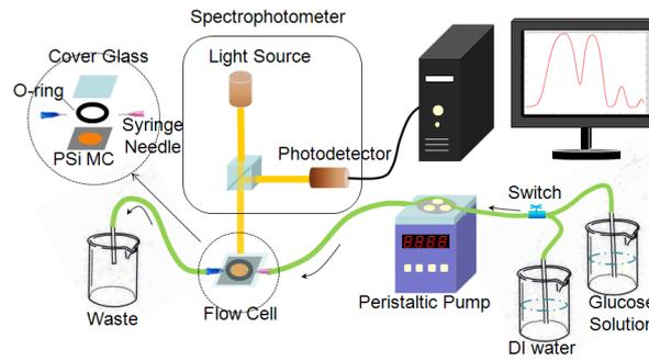
Fig. 1: Schematic view of the intensity-interrogated sensing system. Disassembled flow cell is also shown in the upper-left inset.
