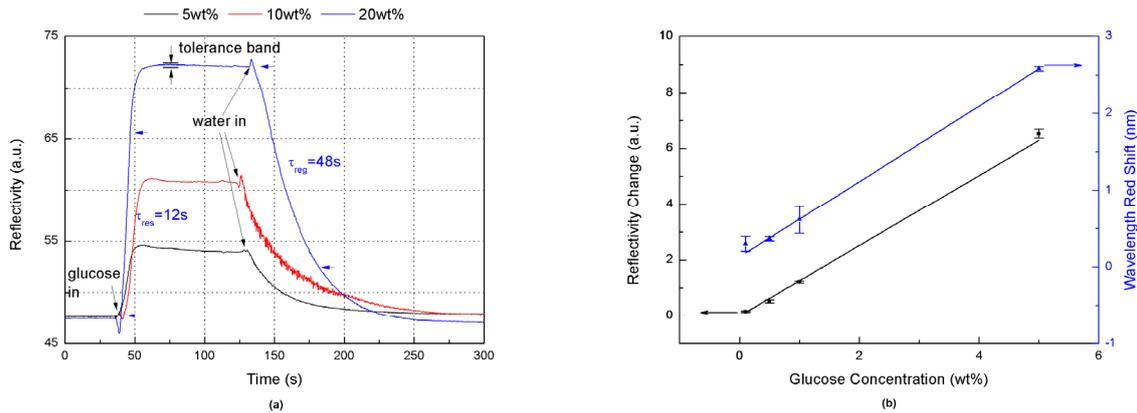
Fig. 3: (a) Intensity-interrogated detection of glucose with a concentration of 5wt%, 10wt% and 20wt% respectively.
