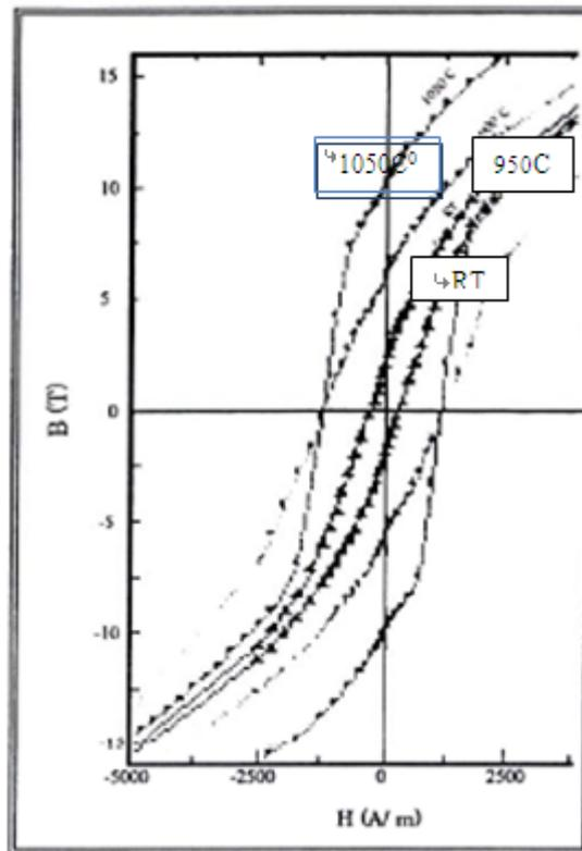
Fig. 4: B-H hysteresis loops of Alnico-5 Alloy at different annealing temperatures
