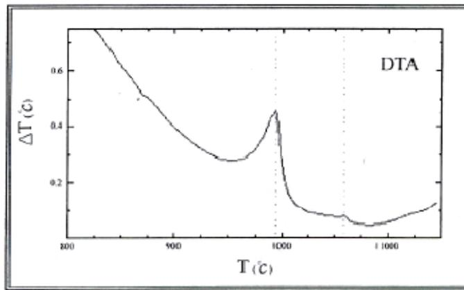
Fig. 3: DTA measurement of Alnico-5 Alloy
