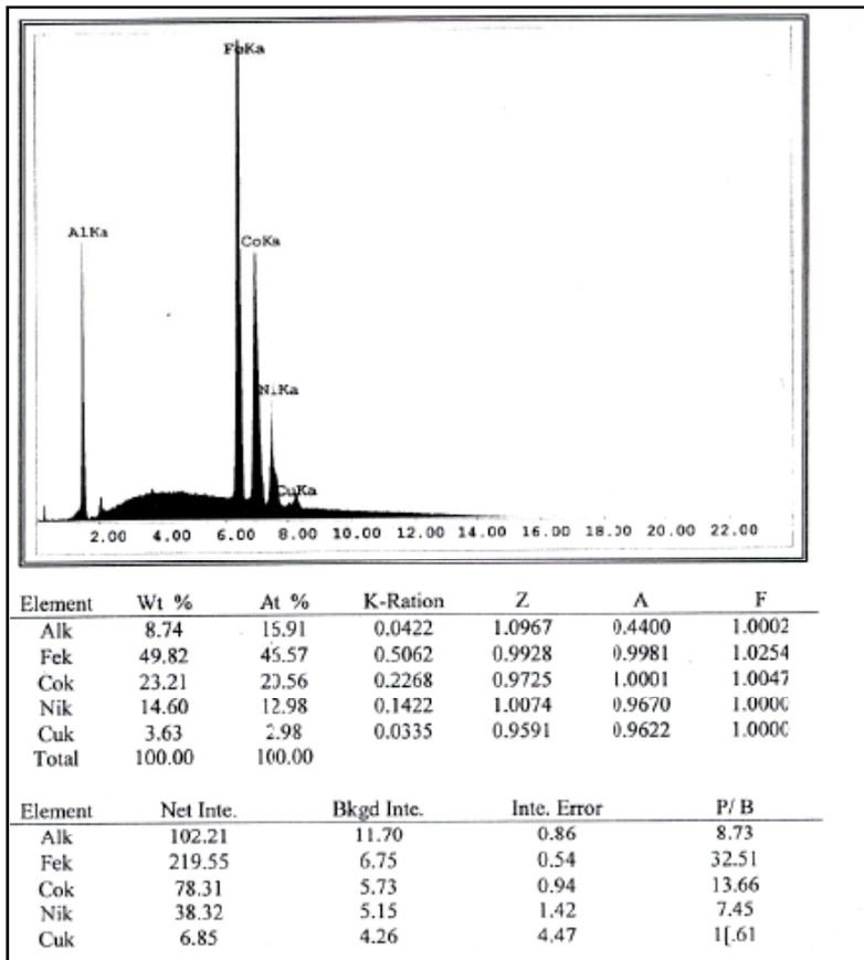
Fig. 1: ESAX for a Alnico-5 Alloy showing elemental spectral peaks
