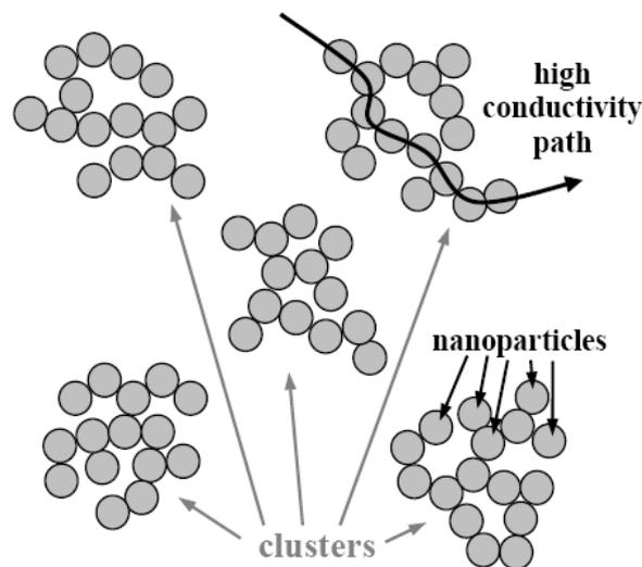
Fig.1: Schematic illustration representing the clustering phenomenon. High conductivity path results in fast transport of heat along large distances.
