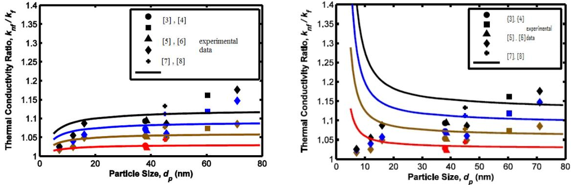
Fig. 2: Comparison of the experimental results of the thermal conductivity ratio for  $\text{Al}_2\text{O}_3/\text{water}$  nanofluid.
