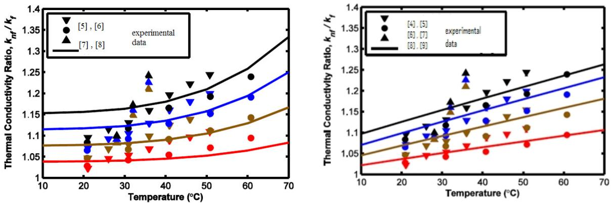
Fig.3: Comparison of the experimental results of the thermal conductivity ratio for  $\text{Al}_2\text{O}_3/\text{water}$  nanofluid.
