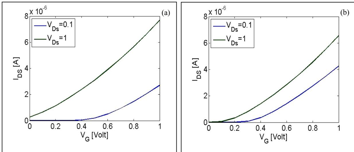
Fig. 4:  $i_{DS}$ - $v_G$  Curves (input characteristic) of CNTFET with (a) simple SWCNT channel and (b)  $\text{NH}_3$  molecules attached to the sidewall of SWCNT channel.
