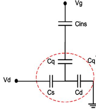
Fig. 1: Capacitive circuit model for the coaxially gated CNTFET [6].
