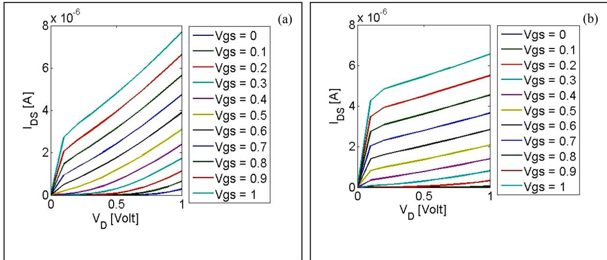
Fig. 3:  $i_{DS}$ - $v_D$  Curves (output characteristic) of CNTFET with (a) simple SWCNT channel and (b)  $\text{NH}_3$  molecules attached to the sidewall of SWCNT channel.
