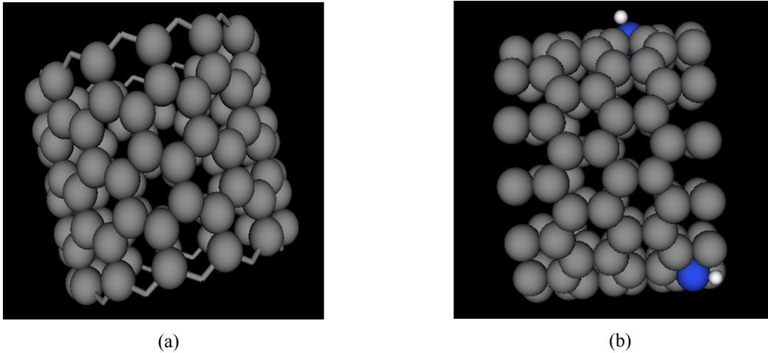
Fig. 2: (a) (13,0) simple SWCNT as a CNTFET channel, (b) (13,0) SWCNT channel of CNTFET with attachment  $\text{NH}_3$  on sidewalls.
