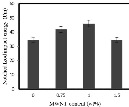
Fig. 3: Izod impact properties of PP and PP/MWNT nanocomposites.
