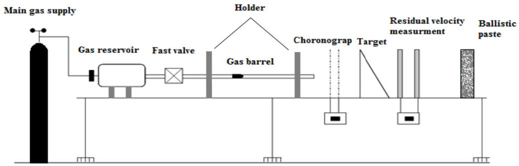
Fig. 1: High velocity impact testing machine (Gas Gun).
