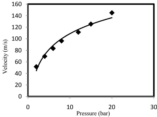
Fig. 2: Projectile velocity calibrations for various helium gas pressures.
