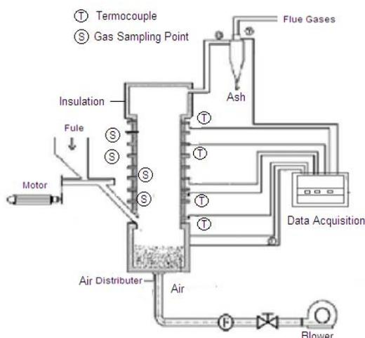
Figure 1. Schematic diagram of the FBC
