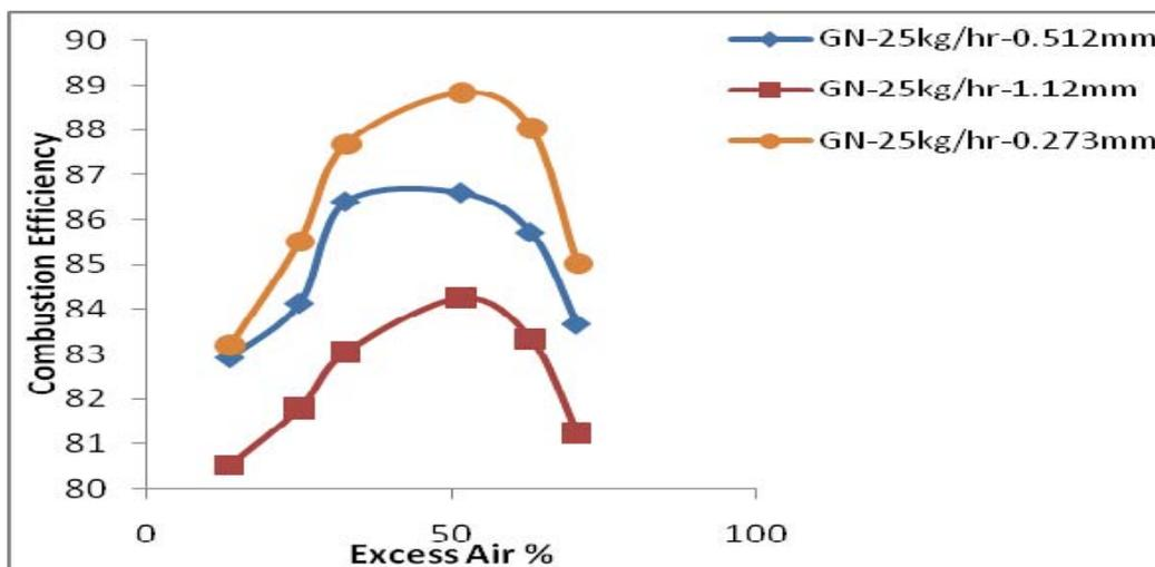
Figure 5. Combustion efficiency of FBC at Different Excess air Factors
