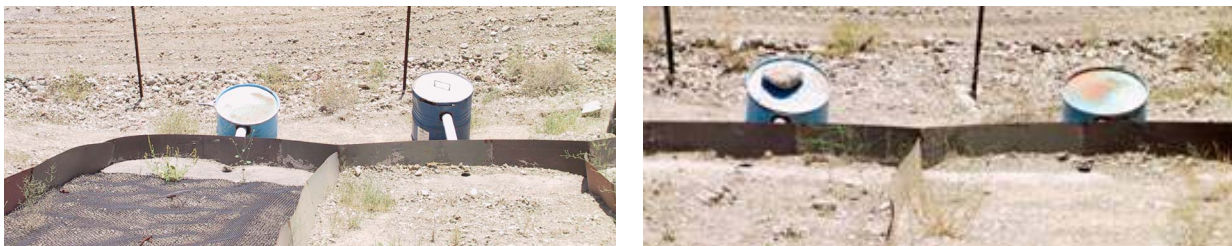
Fig. 2: Sediments produced related to plots with and without geogrid
