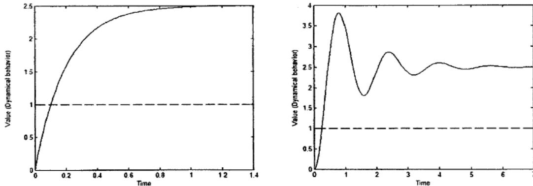
Fig. 2: Output of transformation function in first degree and second degree condition vibration
