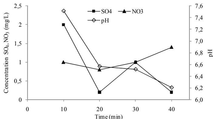
Fig. 2: Variation of  $\text{SO}_4^{2-}$ ,  $\text{NO}_3^-$  concentrations during the rain event on December 27<sup>th</sup> 2010.
