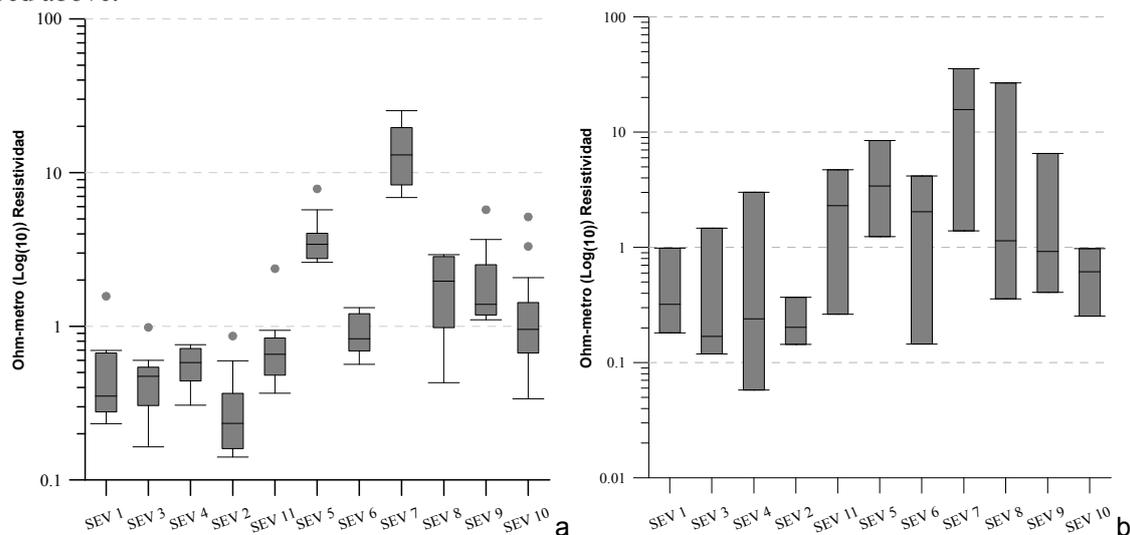
Figure 2. Apparent resistivities (a) and real resistivities (b) recorded in the SEV.
