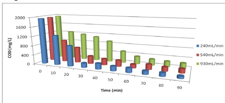
Fig.2: Effect of feed flow rate on COD in semi-continuous flow regime
