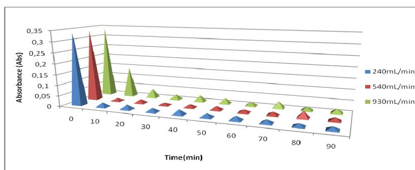
Fig. 3: Effect of inlet flow rate on absorbance in semi-continuous flow regime
