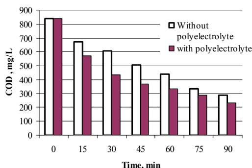
Fig.3: Effect of polyelectrolyte addition on COD concentrations
