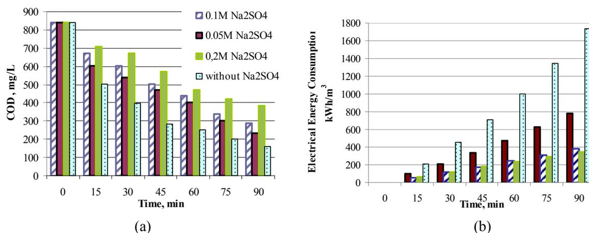
Fig. 2: Effect of supporting electrolyte concentration (a) on COD concentrations and (b) on electrical energy consumptions.
