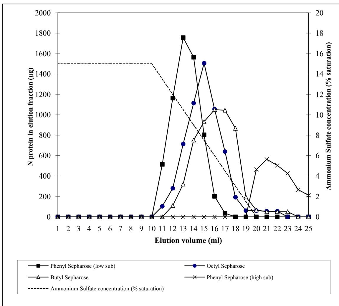
Figure 1 Chromatography of a VLP of NiV on phenyl high sub, phenyl low sub, butyl and octyl Sepharose
