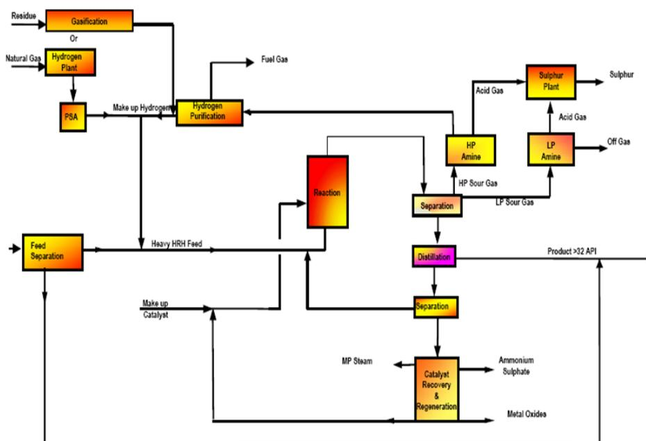
Fig. 3: HRH simplified process flow diagram for heavy crude oil
