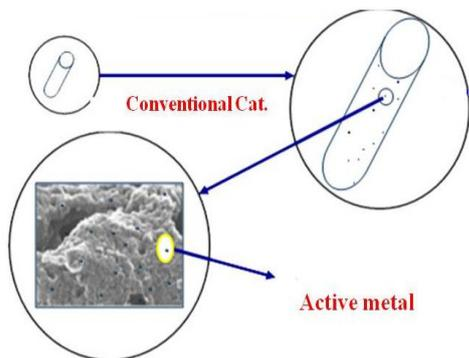
Fig. 1: conventional hydrocracking catalyst particle
