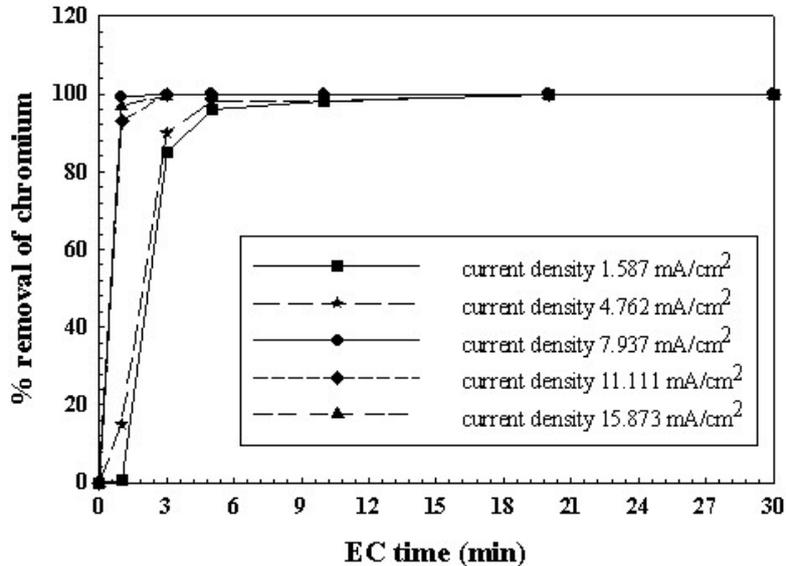
Fig. 2. Influence of different current density in the performance of EC removal of chromium from groundwater using iron electrodes at initial chromium concentration 1 ppm.
