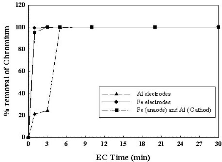
Fig 1. Effluence of types of electrodes in the removal of chromium from groundwater by EC at 0.5 A and initial chromium concentration 1ppm.
