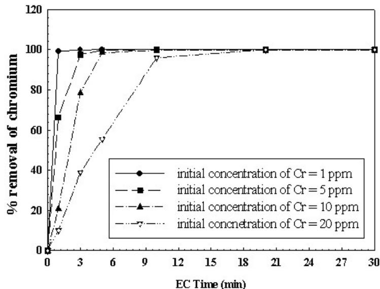
Fig. 3. Influence of different initial concentration in the performance of EC removal of chromium from groundwater using iron electrodes at applied current density 7.9 mA/cm<sup>2</sup> and initial pH 8.
