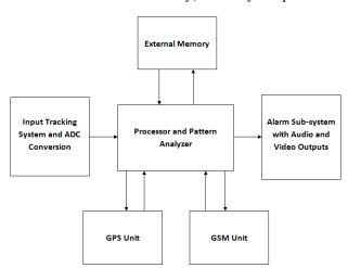
The communication system communicates with the outside world. The GSM module is used for sending relevant data to the doctors or medical practitioners. It's also use to alarm the emergency services in case of any calamity.
