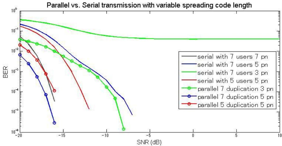
Fig. 7: BER performance comparison according to various spreading code length in case of serial and parallel transmission
