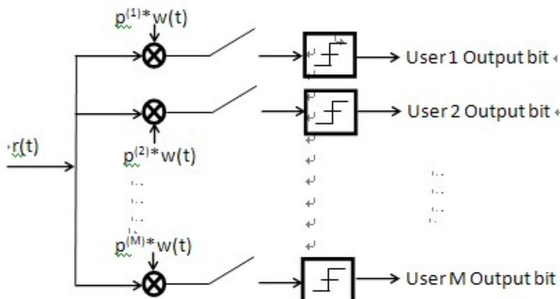
Fig 5: Block diagram of serial receiver
