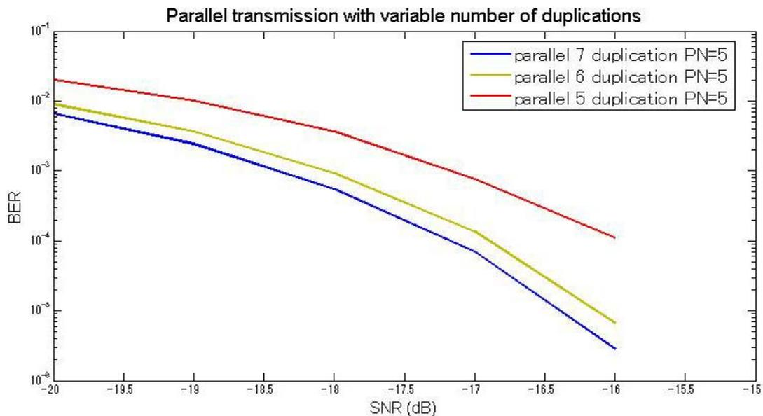
Fig. 8: Parallel transmission with change in number of duplicated bits
