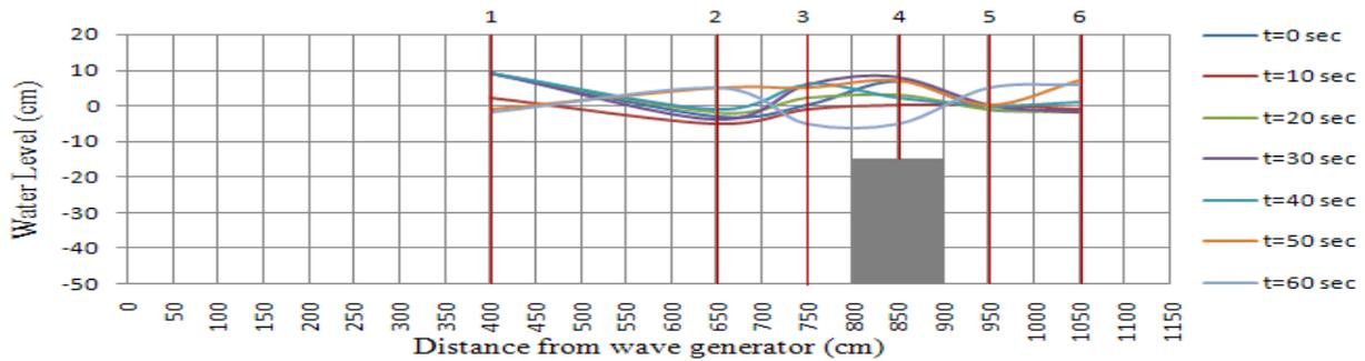
Fig. 3: Water surface profile along the wave flume when  $T=1.6$  sec and  $h_s/d=0.7$
