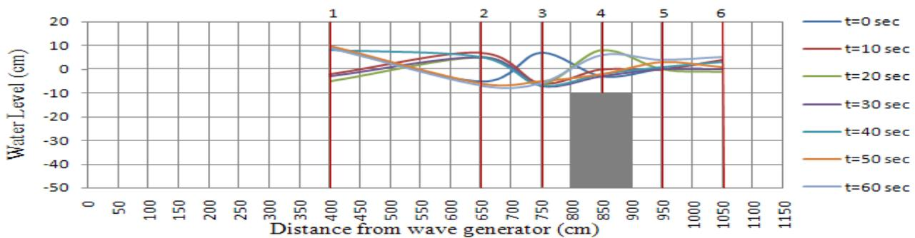
Fig. 4: Water surface profile along the wave flume when  $T=1.6$  sec and  $h_s/d=0.8$
