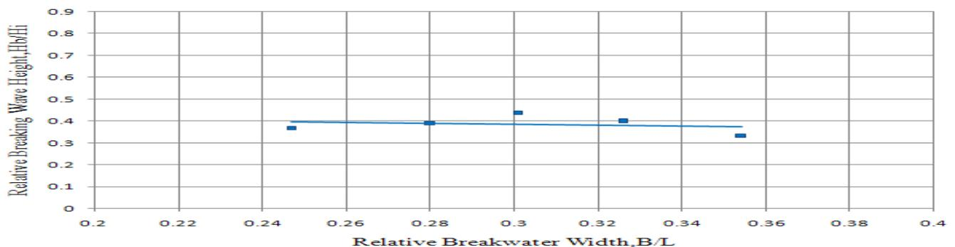
Fig. 7: Effect of relative breakwater width on wave height reduction for  $h_s/d=0.8$
