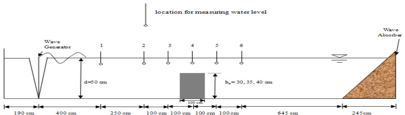
Fig.1: Experimental Set-up
