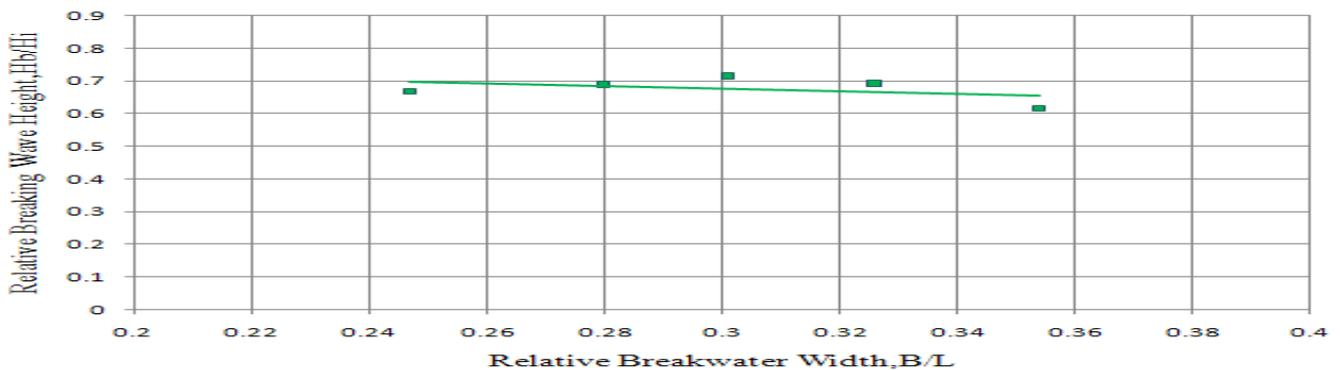
Fig. 6: Effect of relative breakwater width on wave height reduction for  $h_s/d=0.7$
