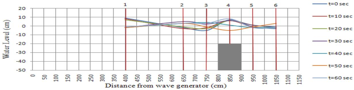
Fig. 2: Water surface profile along the wave flume when  $T=1.6$  sec and  $h_s/d=0.6$
