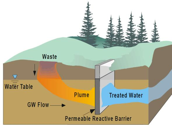
Fig. 1: A Schematic Diagram of Permeable Reactive Barrier
