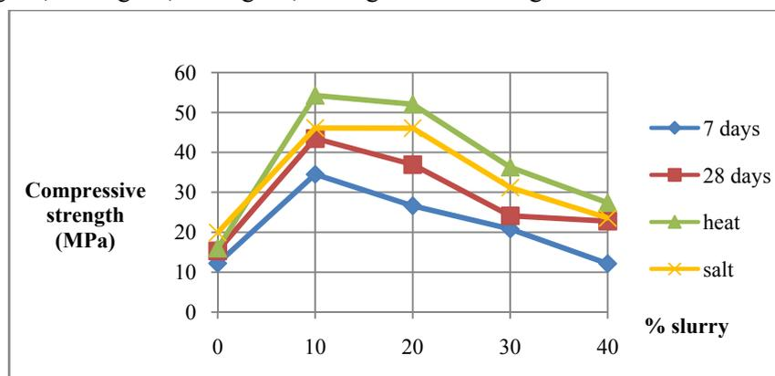
Figure 2: Compressive strength for granite slurry samples
