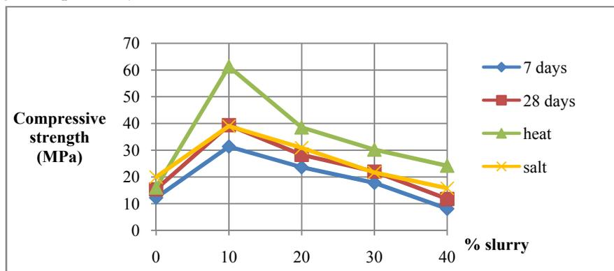
Figure 1: Compressive strength for marble slurry samples
