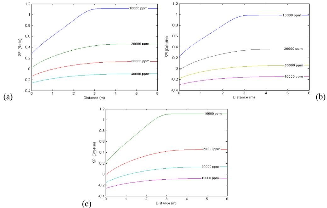
Fig.4. Effect of feed salinity on scaling propensity prediction for (a) Barite precipitation (b) Celestite precipitation (c) Gypsum precipitation.
