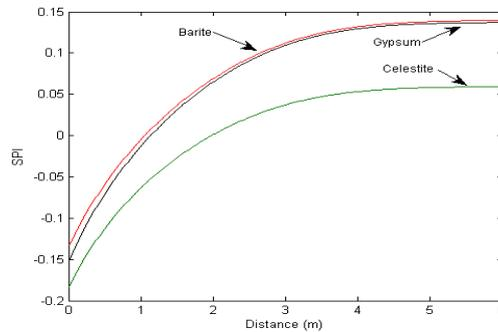
Fig.1. Scaling propensity development for Barite, Celestite and Gypsum precipitation.
