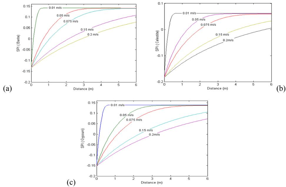
Fig.2. Effect of initial cross flow velocity on scaling propensity development for (a) Barite precipitation (b) Celestite precipitation (c) Gypsum precipitation.
