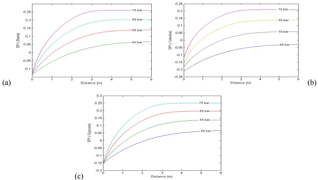
Fig. 3. Effect initial applied pressure on scaling propensity prediction for (a) Barite precipitation (b) Celestite precipitation (c) Gypsum precipitation.
