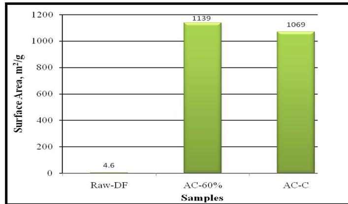
Fig. 3: Single point BET surface area of Raw-DF, AC-60% and AC-C
