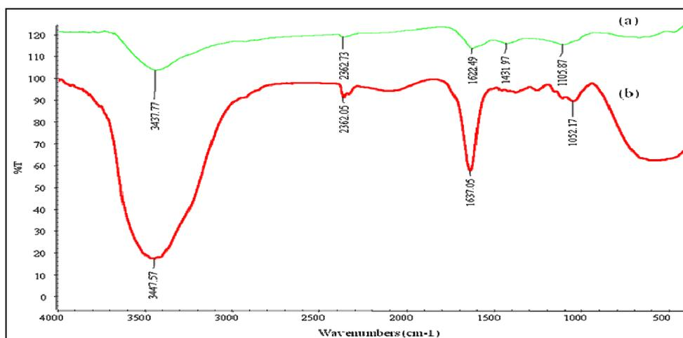
FTIR Spectra for (a) Physical Activation Date Frond, (b) Raw Date Frond
