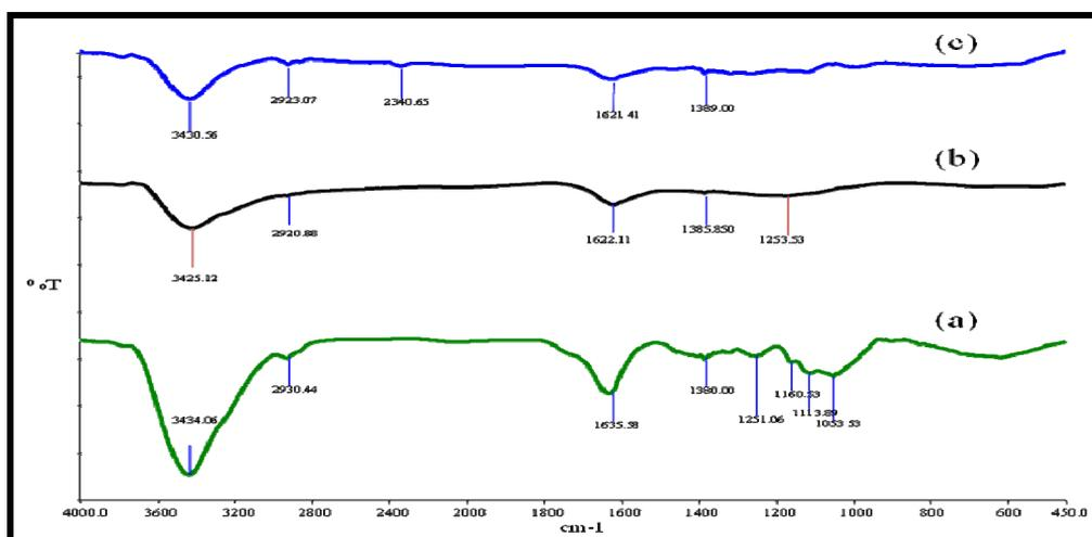
Fig. 2: FTIR Spectra for (a) Raw-DF, (b) AC-60%, (c) AC-C
