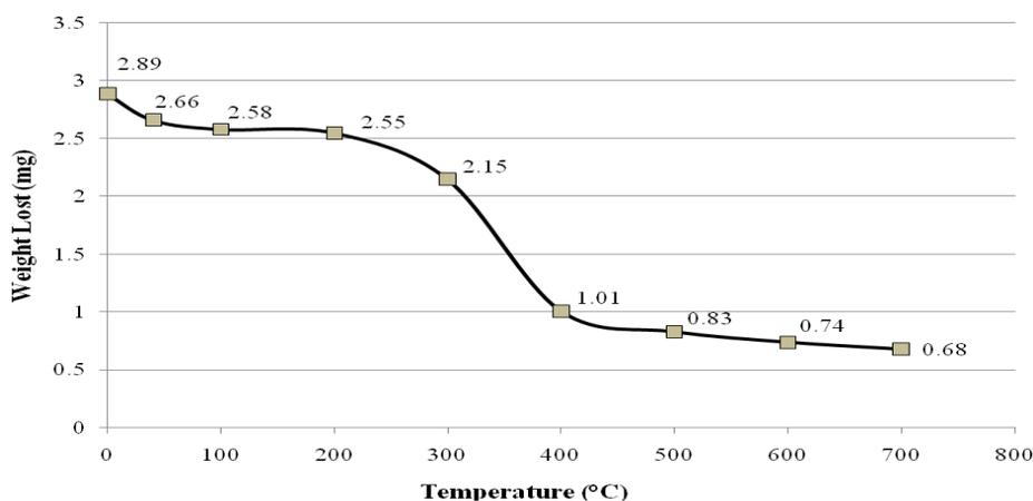
Fig. 1: Thermogravimetric analysis of date fronds
