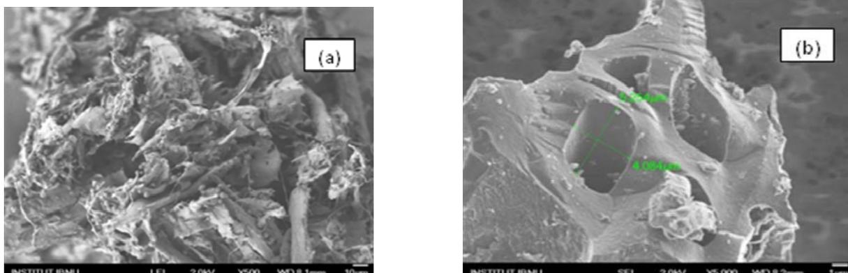
Fig. 4: FESEM of (a) R-PDF and (b) AC-60%  $\text{H}_3\text{PO}_4$  Acid
