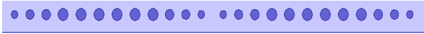
Figure 1. Sketch of the tapered PhC cavity embedded in a PhW waveguide with two mirrors composed by periodically spaced holes and aperiodic taper region inside and outside the cavity. The cavity in SEM picture has 6 holes in each mirror spaced by 350 nm and identical aperiodic taper region inside and outside. The spacings between adjacent holes are 300, 315, and 325 nm respectively. The corresponding hole radii are 65, 80, 85 nm.
