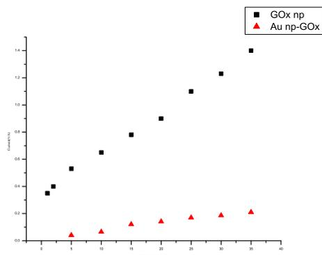
Figure 4. Variation of current as a function of glucose concentration using modified Pt electrode a) *Au-np GOx* Complex ( $\Delta$ ) and b) *GOx-np*( $\square$ ).
