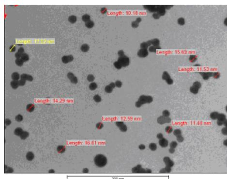
Figure 1. a. Transmission electron micrograph of the Gold nanoparticles (Au np)
