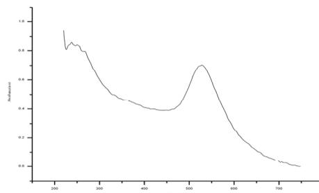
Figure 2. UV-visible absorption spectra of gold nanoparticles
