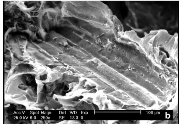
Figure 3. SEM micrograph of the fracture surfaces of composites (a) 5 wt% MAPP (b) 10 wt% MAPP
