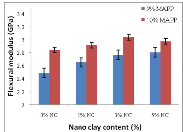
Figure 1. b) Flexural modulus of composites with different amount of nanoclay and MAPP
