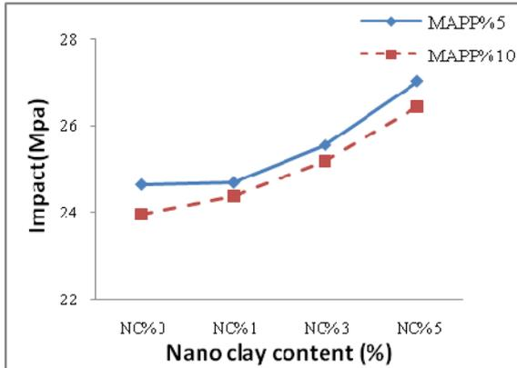
Figure 2. Impact strength of composites with different amount of nano clay and MAPP
