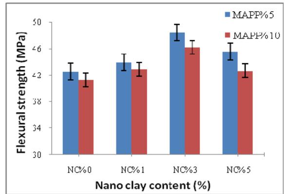
Figure 1. a) Flexural strength of composites with different amount of nanoclay and MAPP
